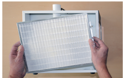
5 Replacing the HEPA Filter
