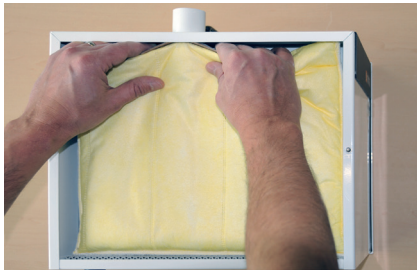
2 Removing the filter bag
