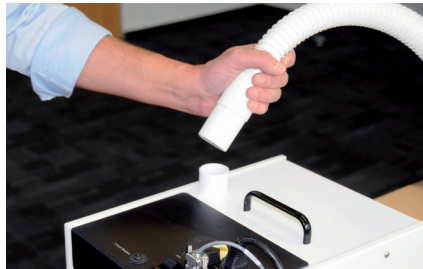
2 Removing and connecting the hoses
