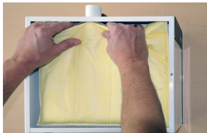
2 Replacing the filter bag
