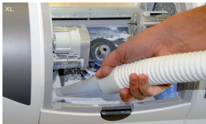
3 Vacuuming the chamber
