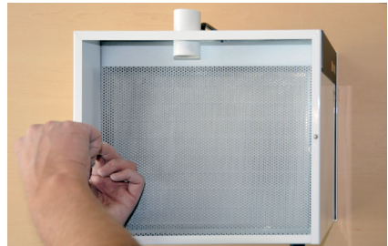
3 Unscrewing the Phillips screws
